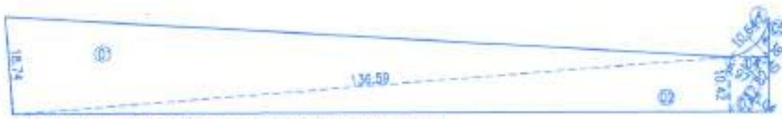
18.00 M. WIDE DRAFT OF ROAD AREA CALCULATION BY TRIANGULATION SCALE-1:500
